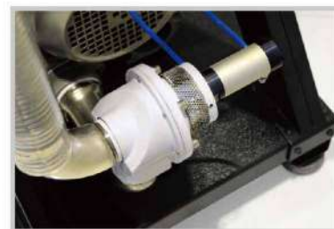
Vacuum breaking valve
