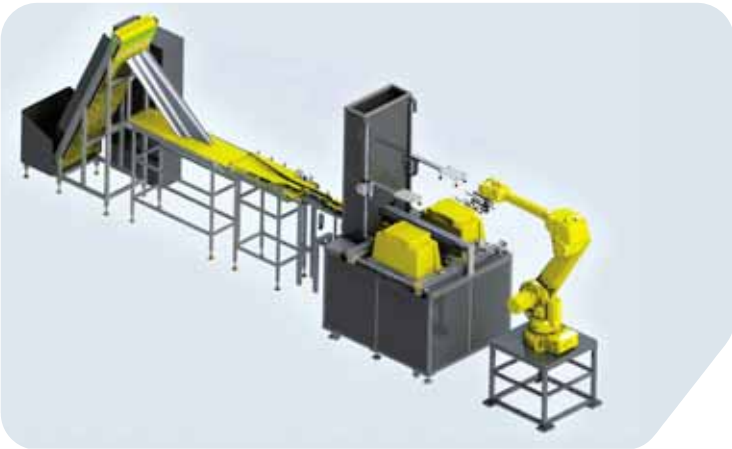
Robot Application (part pick-up, casting insert, assembling, stacking, deburring, degating )
