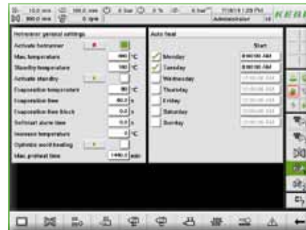
KePlast hot runner setup mask
